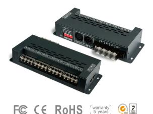
LT-890 DMX CV decoder converts the universal standard DMX512 signal into PWM signal to drive LEDs. works with DMX512 console, 256 grayscale output per channel, 0-100% dimming range with various changing effects. Equiped with DMX standard 3-pin XLR, RJ45 interface, controls single color, two color, RGB LED lights.
